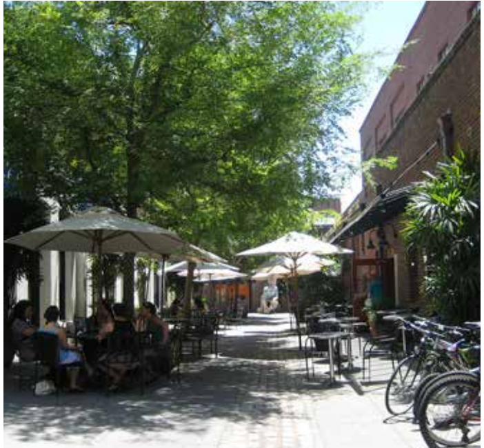
Light coloured paving surfaces reduce solar heat absorption and energy demand, and large trees provide shade and reduce heat island effect
